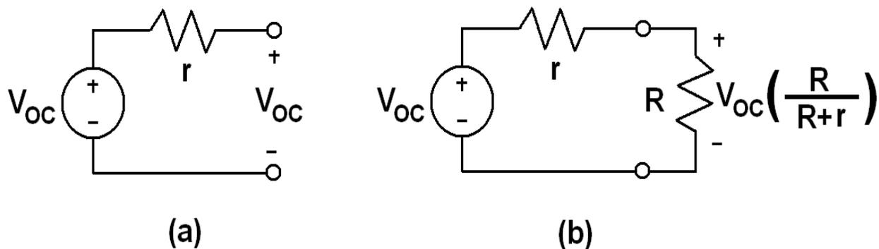
Figure 1 – A Voltage Generation Model (a) No-Load; (b) With Load R
