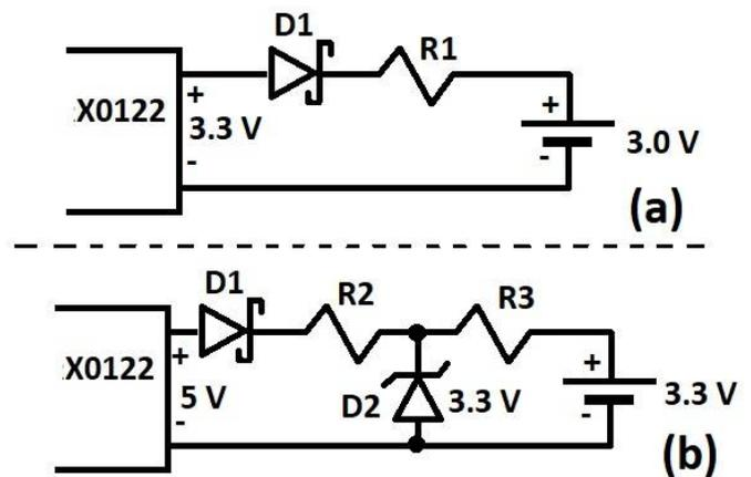
Figure 4 – Two Representative Charging Configurations
