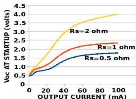
Figure 4 – Voc for Start-up Into a Resistive Load
