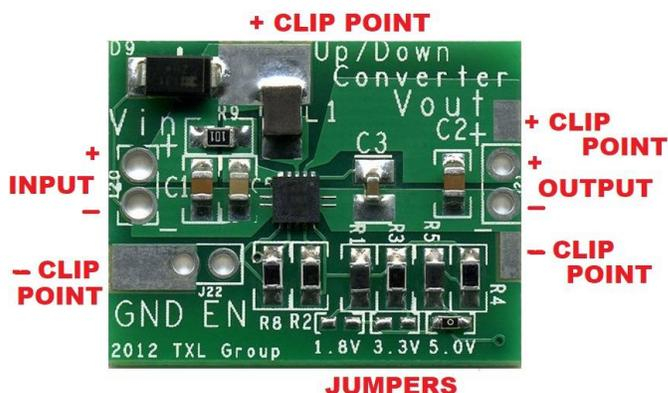
Figure 2 – The X0122 Up/Down Converter
