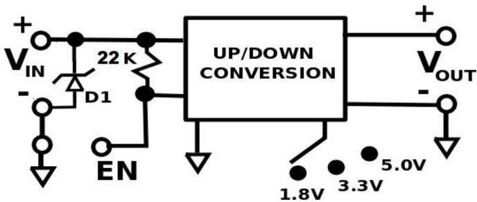
Figure 3 – Electrical Schematic for X0122 Converter
