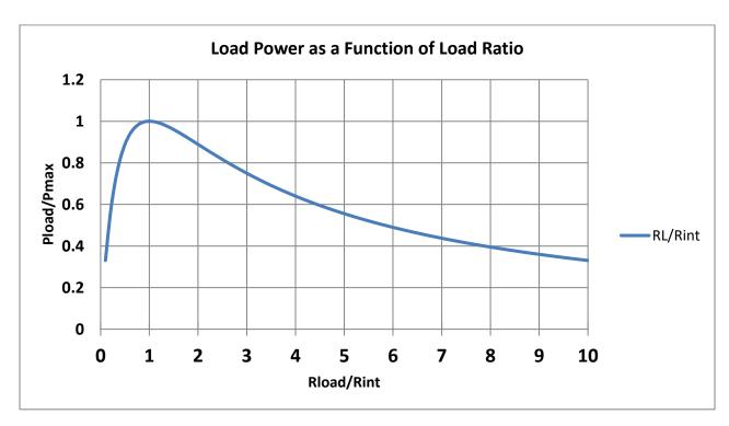
Figure 2 – Output Power as a Function of Load Resistance
