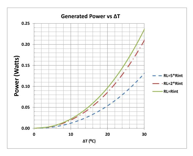
Figure 4 – Load Power as a Function of ∆T for Three Different Load Resistances Using a TXL-199-02Q Module
