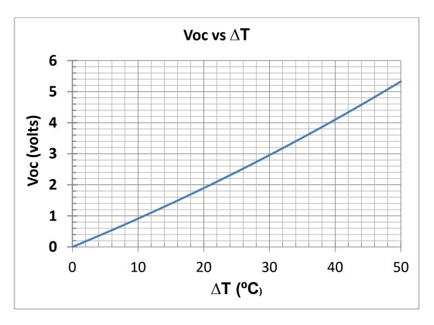
Figure 1 – Open Circuit (No Load) Voltage vs ∆T for the TXL-199-02Q
