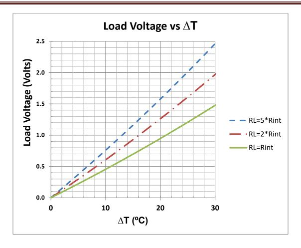
Figure 3 – Load Voltage as a Function of ∆T for Three Different Values of Load Resistance for the TXL-199-02Q
