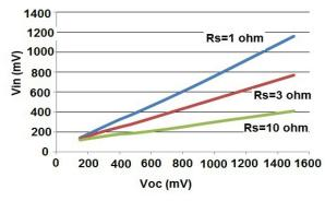
Figure 10 – Vin vs Voc for VB1299 (White)
