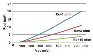
Figure 5 – Power Output vs Voc for VB0410 (Gold)
