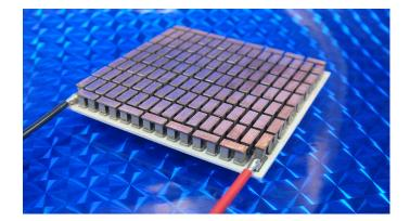
Figure 2 – A 254 Element TE Module (model TXL-127-03L)
