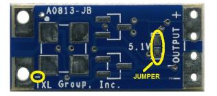
Figure 3 – Jumper Placement on the Backside of the Board to Select 5.1 Volt Regulation
