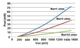
Figure 7 – Power Output vs Voc for VB1299 (White)
