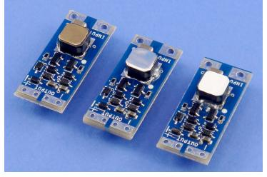
Figure 1 – The VB0410, VB0815 and VB1299 Voltage Boost Bootstrap Converters (Left to Right)
