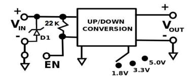
Figure 3 – Electrical Schematic for X0122 Converter
