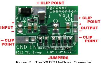
Figure 2 - The X0122 Up/Down Converter
