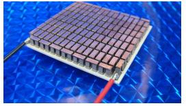
Figure 1 – A 254 Element TE Module
