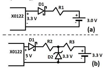
Figure 4 – Two Representative Charging Configurations
